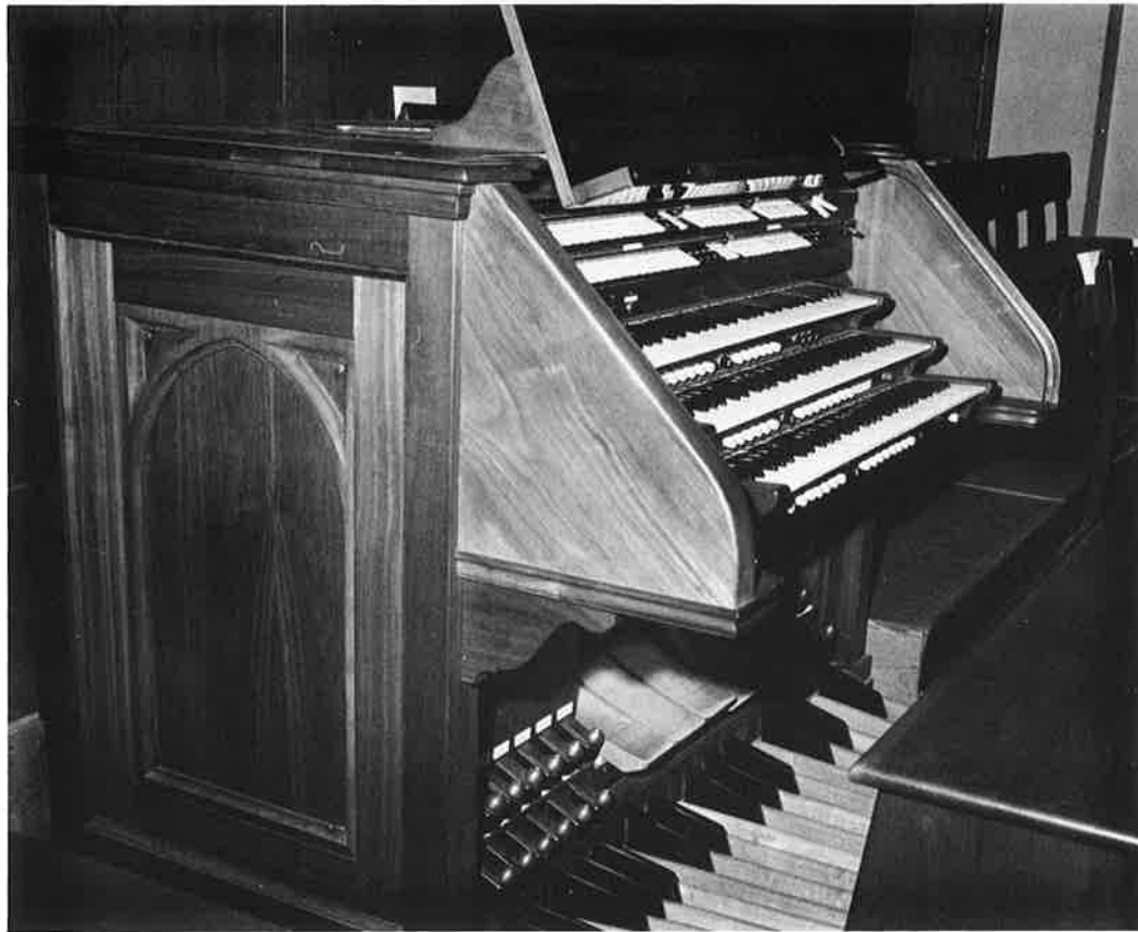
The organ console. Each division (Great, Swell & Brustwerk) has its own keyboard. The Pedalboard is a keyboard played by the organist's feet; the pedal division generally has the deepest pitched pipes. White tablets across the top of the console are stops controlling the various registers or ranks. Buttons and toe studs are adjustable combination pistons for rapid change of stops.
